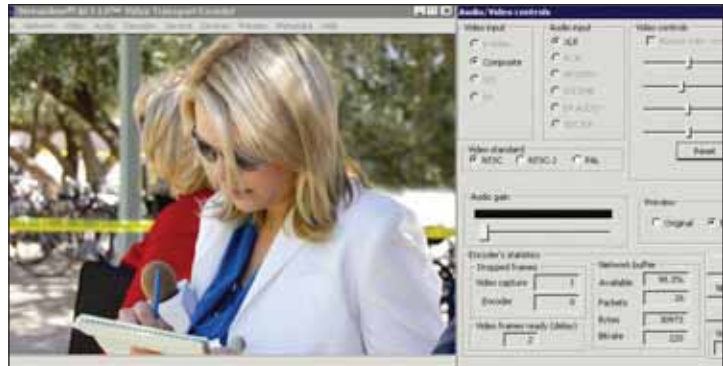
The Streambox ACT-L3 software encoder is used to send live shots from the field to the studio over IP.
